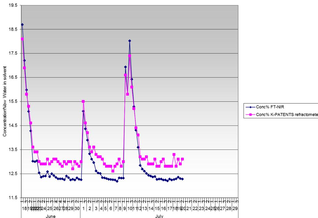
Figure 3. Trend curves for concentration of water in EKC265 plotted with the inline sensors of FT-NIR and refractometer respectively.
