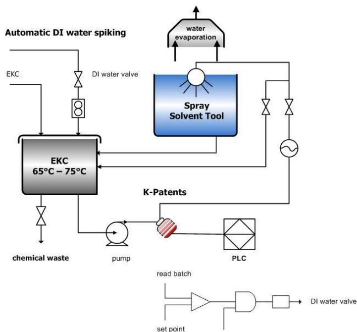
Figure 2. Process schematic of the chemical delivery in a Spray Solvent Tool.
