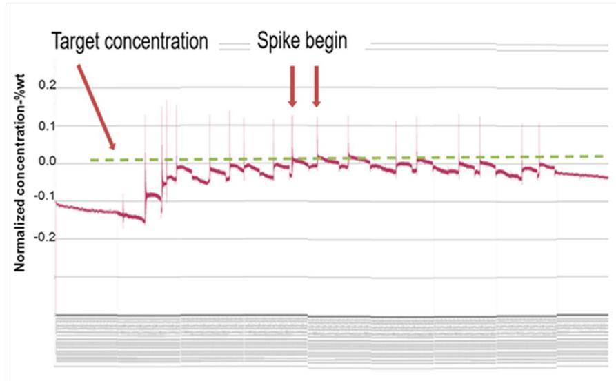
**Fig. 5** Spike function designed in the slurry delivery system to maintain nominal H<sub>2</sub>O<sub>2</sub> concentration in slurry
