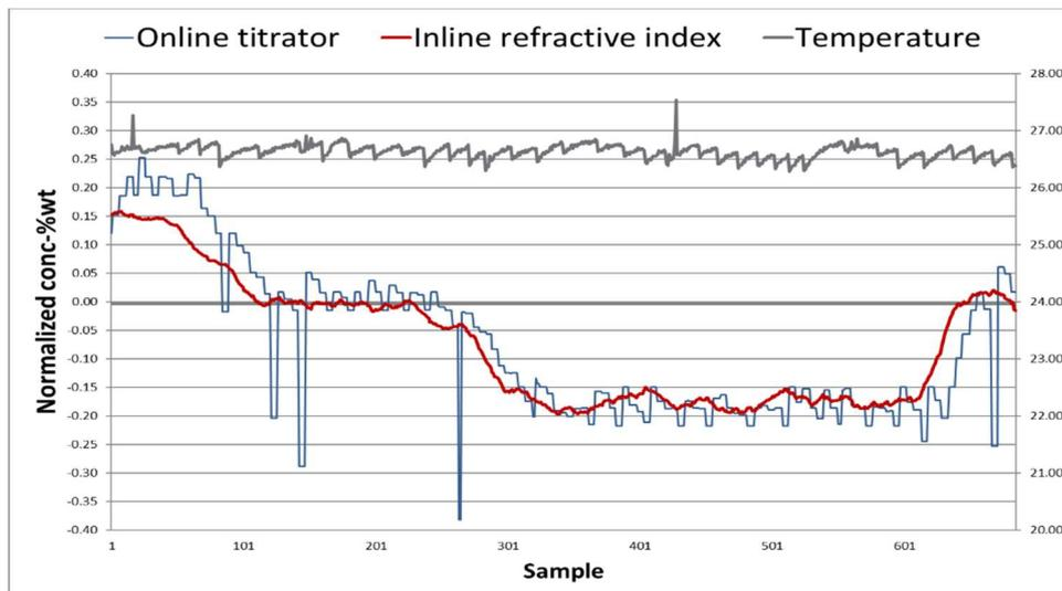
**Fig. 3** Inline refractive index vs. online titration of  $H_2O_2$  in slurry conc%
